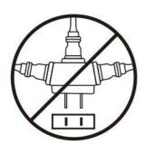
It is forbidden to replace the power cord without authorization, or connect the power cable in the middle and other appliances in parallel.
