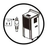
Don't disconnected dehumidifier directly from the power source because it may result in electric shock, fire, etc. Always use the control panel to turn off the dehumidifier. when not in use for a long time shall disconnected the dehumidifier from the power source because dust accumulation may cause leakage, loss, heat, fire, etc.
