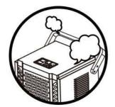
When an abnormal phenomenon (such as a burnt smell) occurs, the operation must be stopped and the power supply turned off. Continued use may result in malfunction, electric shock or fire. Please entrust your local dealer or service outlet for repairs.
