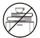
Place the dehumidifier on a stable level surface. If the ground is not flat, it may affect the use of the dehumidifier. Never throw or place anything inside the dehumidifier.
