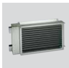
IBW Hot water coil Casing manufactured from galvanised sheet steel. Copper tubes and aluminium fins. Supplied with standard rectangular flanges. Can be fitted in horizontal or vertical position. Maximum water pressure 16bar. Maximum water temperature: 120°C. As accessory: Filtration box and pressure switch to reduce and control the coil clogging.
